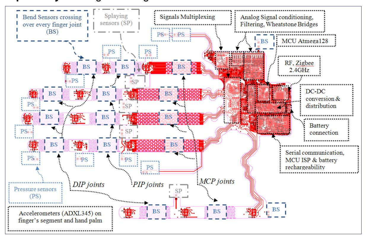
Minimizing the stress under finger flexion, the meander-type structure allows the PCB to undergo large deformations without fracture
