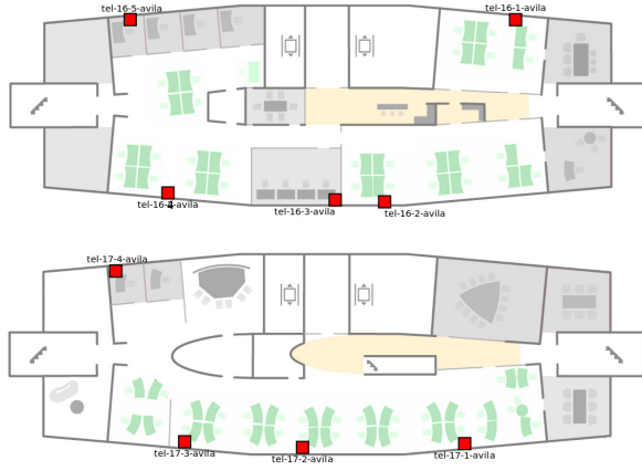
Fig. 1. The BOWL indoor testbed spans two floors. There are five nodes on the 16th floor (top picture) and four nodes on the 17th floor (bottom picture). The host names are indicated with the convention: tel-floor-node .
